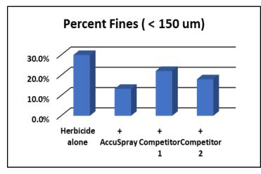
\* Wind Tunnel Study conducted at 24 kph wind at 40 psi. Products applied at 0.25% v/v or 250.0 ml/100L
